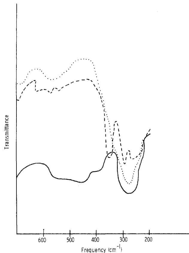
Figure 4. Infrared spectra of (a) \text{ZnCl}_2 (···), (b) \text{ZnCl}_2 \cdot 0.11\text{Et}_2\text{O} (---), and (c) \text{H}_3\text{Zn}_2\text{Cl} \cdot 0.35\text{Et}_2\text{O} (—).
